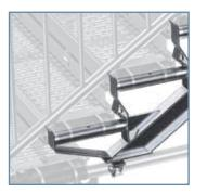
Individual: The lower support of the stair stringer is placed directly on the ledger. This means that the same ledger can be used for all stringer heights. Covered with steel decks or planks for tube hook-up.
